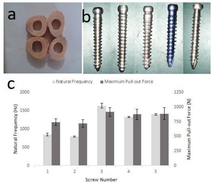
**Fig. 1.** a) Divided cortical bovine samples from tibial portion, b) Screw samples with different thread distribution and specification mostly different in core shape, crest thickness and self-tapping feature, and c) Natural frequency and maximum pull-out force versus every screw number based on the table 1.
